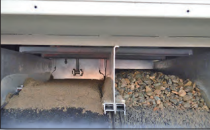
PESATURA INERTI WEIGHING OF AGGREGATES
